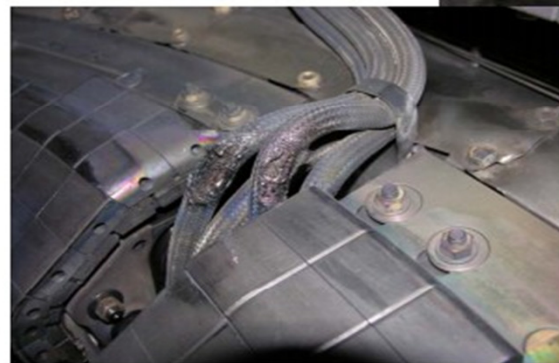
“Far away” diagnostic harness burned/melted by runaways
